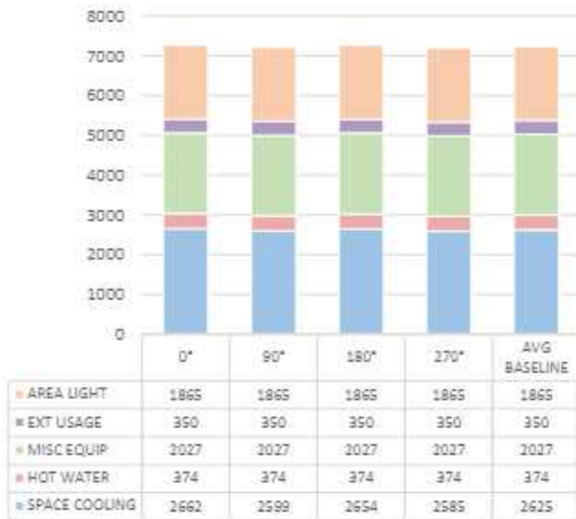
ENERGY-USE COMPARISON FOR ALL END USES BASELINE CASE (MWh) - As per ECBC 2007
