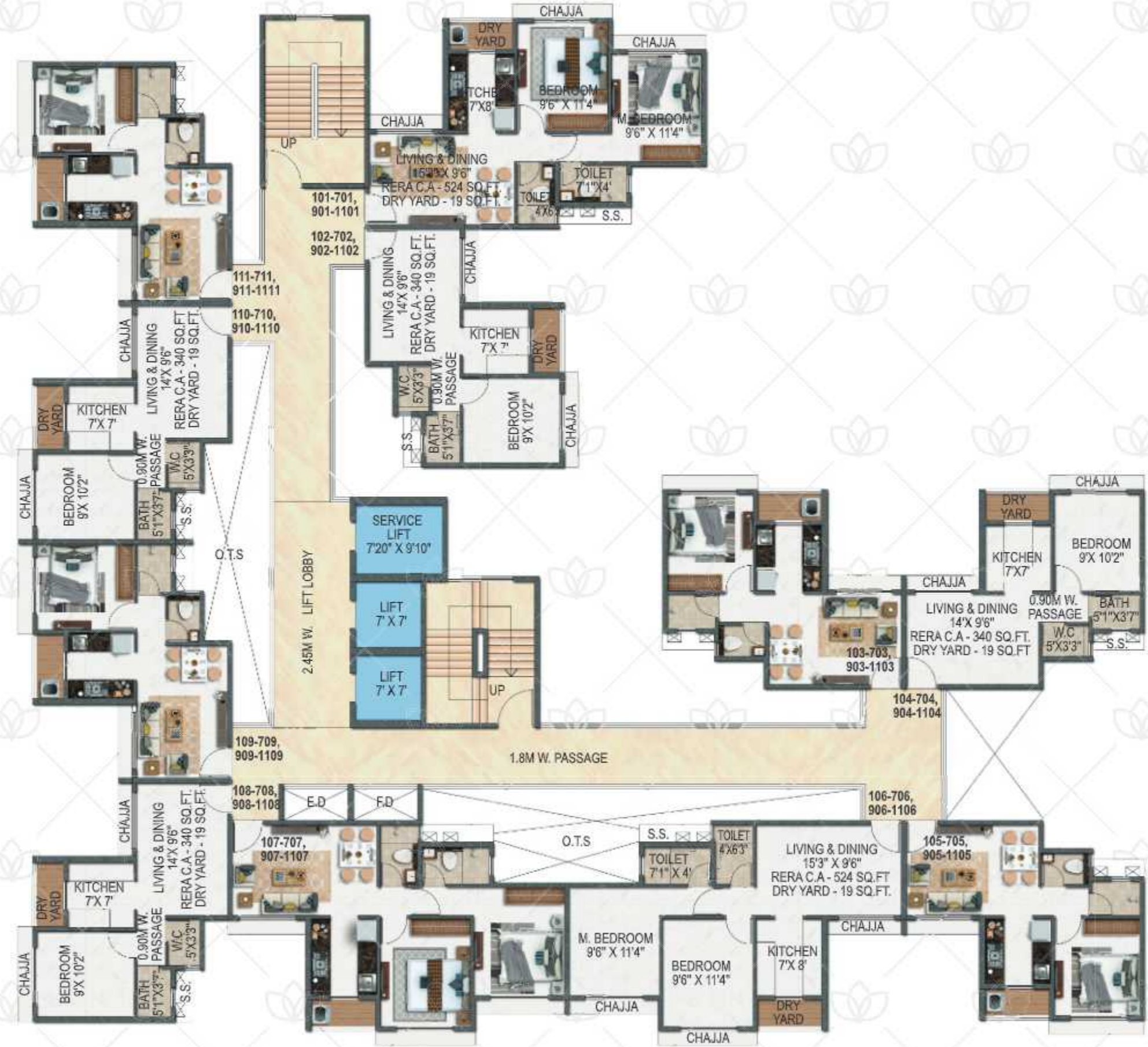
TYPICAL 1 ST TO 7 TH & 9 TH TO 11 TH FLOOR PLAN - BUILDING NO.1 (WING B)
