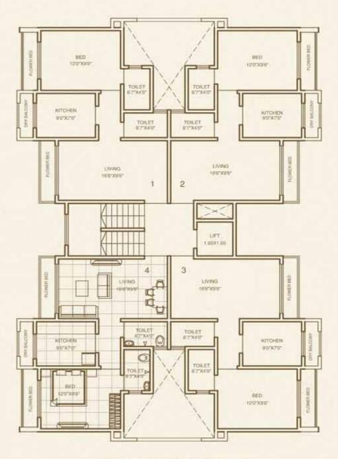
TYPICAL FLOOR PLAN (1ST TO 7TH)
